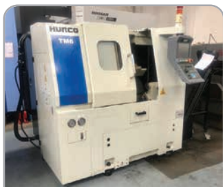
Hurco TM6 2-Axis CNC Lathe with WinMax control, 8" power chuck, tailstock, swarf conveyor. YOM 2008
