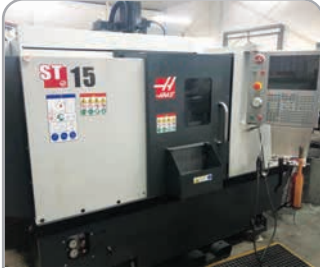
Haas ST15-TCE with power chuck, tailstock, swarf conveyor, parts catcher. YOM 2018
