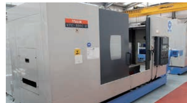
Mazak VTC 300C II vertical machining centre , PC Fusion 640M CNC, BT40, speeds to 12000rpm, swarf conveyor, handwheel, 2000 x 760mm table, X=1760 Y=760 Z=660mm (20954) £P.O.A Email: nick@newcentury.co.uk
