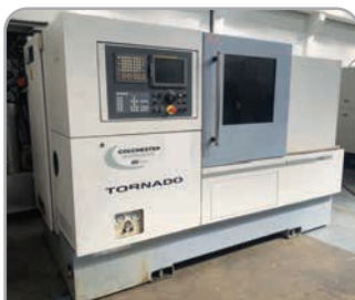
Colchester T8M with Fanuc control, driven tools, C-axis, tailstock & tooling YOM 2008
