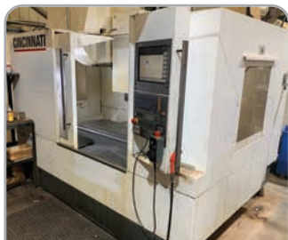
Cincinnati Lamb CFV 800i with Heidenhain i530 control, 30-tool ATC, Nikken 4th axis, 12,000RPM spindle with through coolant. YOM 2008
