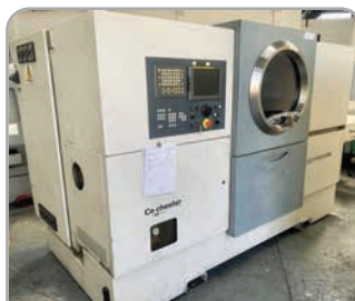
Colchester T8 CNC Lathe with Fanuc control, 210mm dia chuck, 77.5mm bore, parts catcher & swarf conveyor. YOM 2008
