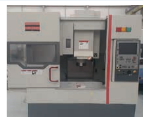
Quasar MV154 E vertical machining centre , New 2010, Heidenhain TNC620 CNC, speeds to 12000rpm, BT40 , 30 ATC, 900 x 500mm table, X=700 Y=530 Z=560mm (20986) £P.O.A Email: nick@newcentury.co.uk
