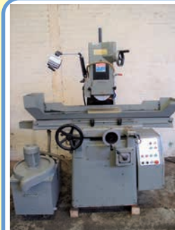
SEEDTEC YSG-618AHR Surface Grinder , (1993), Capacity 500 x 150mm, Travels 550 x 177mm, Magnetic chuck 340 x 150mm, Auto reversing saddle, Coolant and dust, Excellent condition. Email: sales@ronthompsonmachinery.co.uk
