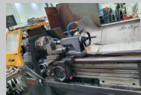
In Very good condition.....POA C/w 3 & 4 jaw chucks, Two axis dro, Q'change toolpost & holders, Lo-vo-lite, bedstop. Original slideways very good & very good headstock.
