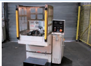
SUNNEN SSH-1680 HONE New 2018, Bore 3 - 60mm, Max Bore Length 250 mm, Spindle Speeds 250-2500rpm, Stroke speed 80-310spm C/w light guards
