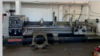
Colchester Magnum 1250 x 3m Gap bed lathe £15,500+vat C/w 3 & 4 jaw chucks, one axis dro, light & heavy duty steady, Travelling steady, Q'change toolpost & holders, Taper turner, plus lots of extra tooling. Quiet headstock & good slides. Rapid feed button needs replacing. This lathe can be seen under power at a client's workshop.
