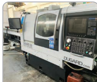
Dugard 32 Sub-Spindle Sliding Head Lathe with Syntec PC control, driven tools, 3m bar feed, tooling. YOM 2010
