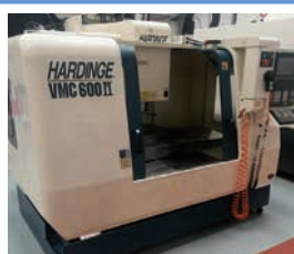
Hardinge VMC 600 vertical machining centre , Siemens 810D CNC, BT40, speeds to 8000rpm, 20 station toolchanger, 750 x 510mm table, X=600 Y=510 Z=510mm (20984) £P.O.A Email: nick@newcentury.co.uk
