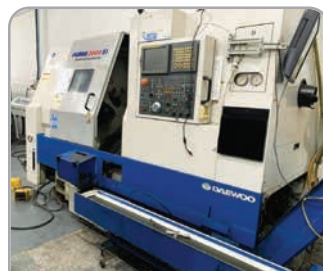
Daewoo Puma 200SY with Fanuc control, sub spindle, driven tools & 2x C-axis, bar feed & swarf conveyor. YOM 2006
