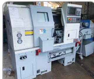
XYZ CT52 with Siemens 828D control & Shopturn, 16C collet adaptor & 8" power chuck, tailstock, swarf conveyor. YOM 2012
