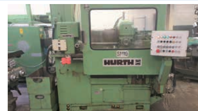
HURTH KF32a Automatic Twin Spindle Spline Milling Machine , Table size 1500 x 375mm, Horizontal travel of spindle head 400mm, Max. component length 550mm. Twin spindle index head, Hydraulic tailstocks, Arbor support, late machine. Email: sales@ronthompsonmachinery.co.uk
