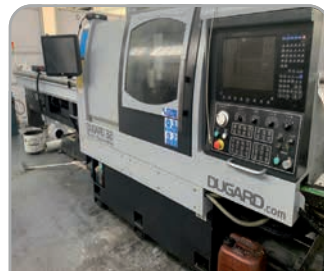
Dugard 32 Sub Spindle, Syntec PC controlled 32mm cap sliding head lathe with 3 metre barfeed, driven tools C-Axis x 2. YOM 2011
