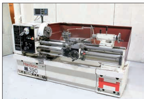
Harrison M390 x 1250mm Gap Bed Centre Lathe with DRO
