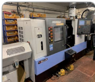
Doosan Puma 280M with Fanuc control, driven tools & C Axis, barfeed & swarf conveyor. YOM 2008
