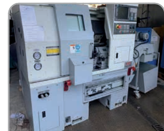
XYZ CT52 with Siemens 828D control & Shopturn, 8" power chuck, 16C collet adaptor, parts catcher, tailstock, swarf conveyor YOM 2012
