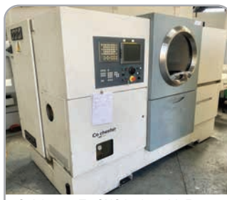
Colchester T8 CNC Lathe with Fanuc control, 210mm dia chuck, 77.5mm bore, parts catcher & swarf conveyor. YOM 2008
