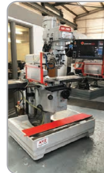
XYZ SMX 2000-2 with R8 spindle, power draw bar, DXF file reader and table guards. YOM 1996
