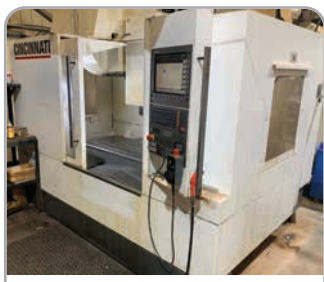
Cincinnati Lamb CFV 800i with Heidenhain i530 control, 30-tool ATC, Nikken 4th axis, 12,000RPM spindle with through coolant. YOM 2008
