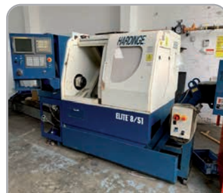
Hardinge Elite 8/52 with Fanuc control, C-axis & live tools, driven tooling package, bar feed. YOM 2003
