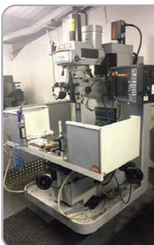
XYZ SMX 2500 with ProtoTrak SMX control, vari-speed R8 taper spindle, electronic handwheels, power drawbar. Immaculate! YOM 2015
