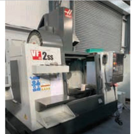
Haas VF2SS with 4th axis drive, 12,000RPM spindle, direct drive spindle, 24-tool rapid ATC. YOM 2010
