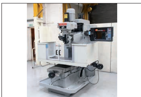
2015 XYZ SMX 3500 Bed Mill. 787mm X Travel
