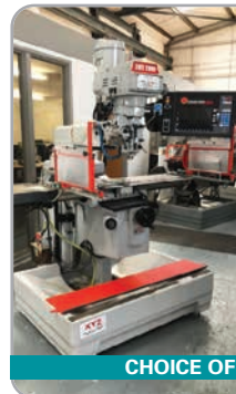
XYZ SMX 2000-2 with R8 spindle, power draw bar, DXF file reader and table guards. YOM 2016
