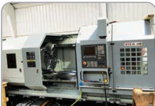
XYZ XL 1100 x 2m with Siemens control, 1,000mm 4-jaw, 160mm spindle bore, 1,100mm swing, auto indexing tool post, power tailstock. Virtually unused! YOM 2019
