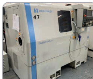
Hardinge Talent 645-SV with Fanuc control, 6" chuck, 42mm spindle. Immaculate! YOM 2006
