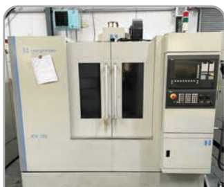
Hardinge Bridgeport XV 710 with Siemens 810D control & Shopmill, 8,000RPM BT40 spindle. Immaculate! YOM 2007
