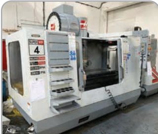
Haas VF4SS with 4th axis drive, 12,000RPM spindle, direct drive spindle, 24-tool rapid ATC. YOM 2008
