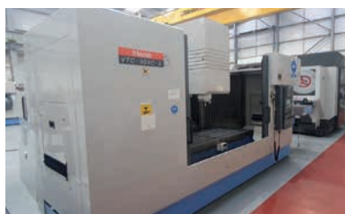
Mazak VTC 300C II vertical machining centre , PC Fusion 640M CNC, BT40, speeds to 12000rpm, swarf conveyor, handwheel, 2000 x 760mm table, X=1760 Y=760 Z=660mm (20953) £P.O.A Email: nick@newcentury.co.uk
