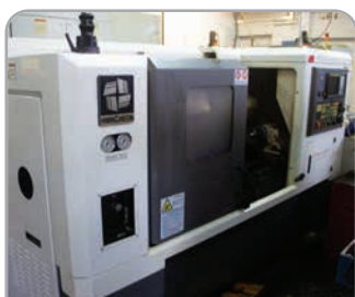
Hwacheon Hi-Tech 200Ai with Fanuc control, 8" chuck, tailstock, parts catcher, removable tool probe. YOM 2005
