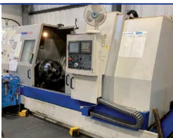
Daewoo Puma 500 CNC Lathe Year: 2002 / FANUC 18i-T control (ST3441)
