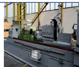
Herkules Heavy Duty Cylindrical Grinder Capacity: 915 x 3200mm (ST3061)
