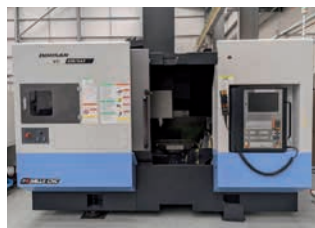
Doosan VC630 / 5AX vertical machining centre , Installed 2017, Heidenhain TNC 630i CNC full 5 axis, BT40, speeds to 12000rpm, X= 650 Y=765 Z=520mm A=150 +30 - 120 deg(20996) £P.O.A Email: nick@newcentury.co.uk
