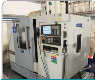
XYZ VMC 710 with Siemens 828D control, 24-tool side-mount ATC, 8,000RPM. 2010 & 2014
