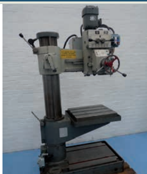
Qualters & Smith R2 24" 3MT Radial Arm Drill
