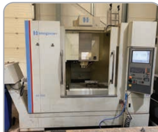
Hardinge Bridgeport XR 1000 with Heidenhain i530 control, 12,000RPM direct-drive spindle, thru coolant, 4th axis probing. YOM 2010
