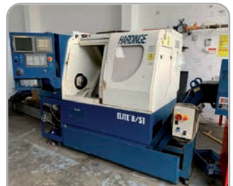
Hardinge Elite 8/52 with Fanuc control, C-axis & live tools, driven tooling package, bar feed. YOM 2003
