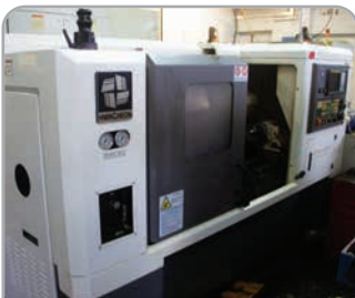
Hwacheon Hi-Tech 200Ai with Fanuc control, 8" chuck, tailstock, parts catcher, removable tool probe. YOM 2005
