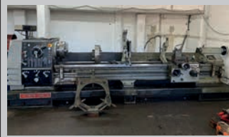
Colchester Magnum 1250 x 3m Gap bed lathe £15,500+vat C/w 3 & 4 jaw chucks, one axis dro, light & heavy duty steadies, Travelling steady, Q'change toolpost & holders, Taper turner, plus lots of extra tooling. Quiet headstock & good slides. Rapid feed button needs replacing. This lathe can be seen under power at a client's workshop.
