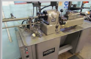
Second operation capstan Lathe with Barfeed £POA
