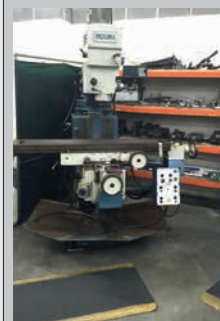
Heavy Duty Induma Vertical Mill. Table 60" x 11". ISO 40int. Two axis Anilam dro. Variable speed head. Variable & Rapid feed to table. Coolant £2,500+VAT
