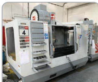
Haas VF4SS with 4th axis drive, 12,000RPM spindle, direct drive spindle, 24-tool rapid ATC. YOM 2008
