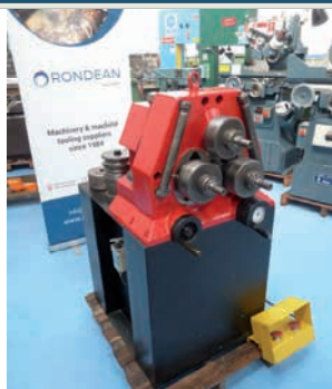
Tauring Alfa 40 3 driving rolls with tooling
