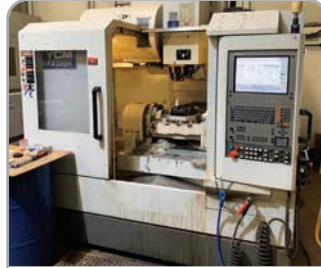
YCM FX 350A 5-Axis Machining Centre with Heidenhain i530 control, 12,000RPM, thru coolant, 60-tool ATC, glass scales & probing. YOM 2012
