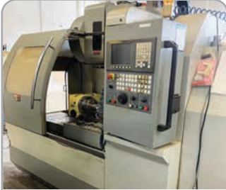
Leadwell V-40 VMC with Fanuc control, 8,000RPM spindle & Nikken 4th axis head. YOM 2006
