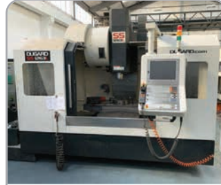
Dugard SS1263L VMC with Heidenhain i530 control 12,000RPM direct-drive spindle, thru coolant, 1,200kg sd table load. YOM 2015
