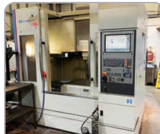
Hardinge Bridgeport XR 760 with Heidenhain i530 control, 12,000RPM direct-drive spindle, thru coolant, 4th axis probing. YOM 2008
