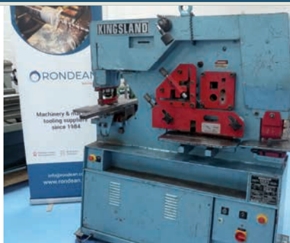
Kingsland 55 ton 2 Operator Steelworker
