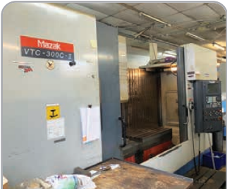
Mazak VTC 300-C Travelling Column VMC with Mazatrol PC Fusion control, 12,000RPM spindle. YOM 2004
