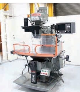
XYZ 1500 3 Axis CNC Turret Milling Machine ProtoTRAK Control
