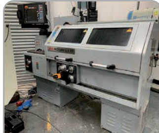
XYZ SLX 355 with ProTrak SLX control, 3 jaw chuck, Traking, quick change tool post YOM 2014
