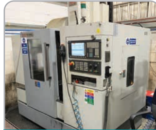
XYZ VMC 710 with Siemens 828D control, 24-tool side-mount ATC, 8,000RPM. 2010 & 2014
