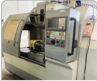
Leadwell V-40 VMC with Fanuc control, 8,000RPM spindle & Nikken 4th axis head. YOM 2006
