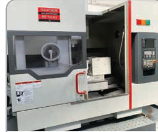
Quaser MF500-C 5-Axis Trunnion Style VMC with Siemens 828D control, 12,000 RPM, 30 tools. Immaculate! YOM 2012
