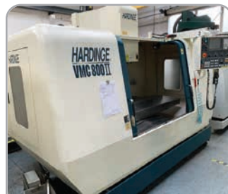
Hardinge VMC 800 Sr II with Fanuc 0i control, 8,000RPM, 20-tool ATC. YOM 2003
