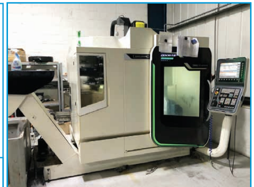
DMG DMU50 Ecoline (2014). 12k spindle, ISO 40, 30-tool T/C, 3+2 machining with Siemens 840D control
