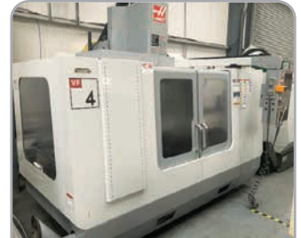
Haas VF4, 1,270mm x 508mm x 635mm movements, 8,100RPM, swarf auger. YOM 2007
