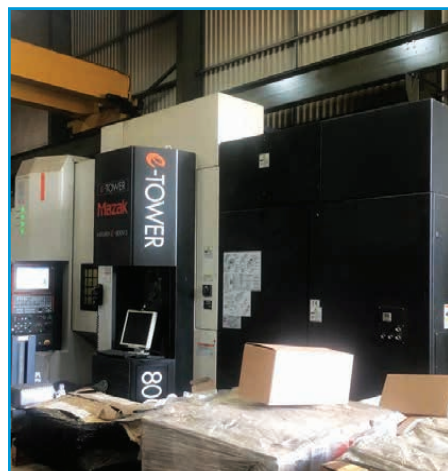
2008 MAZAK Integrex 800V/5 II E Tower . B-axis movement head: +120/-30°, Mazak Matrix control, max machining dia 730mm, maximum workpiece weight 680kg, rapid feedrates 50m/min, spindle speed 12,000rpm (milling), 80 ATC, traverses XYZ: 1,100/800/900mm, through-spindle coolant, tool setter, swarf conveyor, twin-pallet, full 5-axis machine, the table spins just like a lathe to machine large components in one set-up
