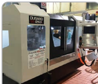
Dugard SS1263L VMC with Heidenhain i530 control 12,000RPM direct-drive spindle, thru coolant, 1,200kg sd table load. YOM 2015
