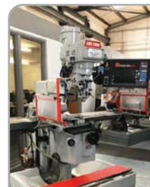
XYZ SMX 2000-2 with R8 spindle, power draw bar, DXF file reader and table guards. YOM 2016
