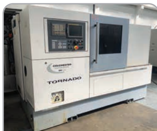
Colchester T8M with Fanuc control, driven tools, C-axis, tailstock & tooling YOM 2008
