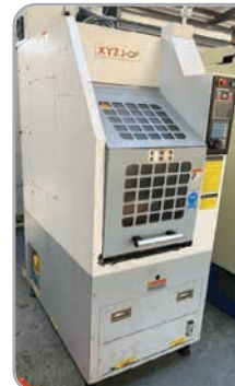
XYZ 2 OP portable VMC with ProtoTrak control, 8-tool ATC & tooling. YOM 2016
