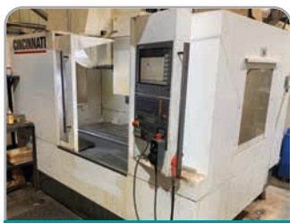
Cincinnati Lamb CFV 800i with Heidenhain i530 control, 30-tool ATC, Nikken 4th axis, 12,000RPM spindle with through coolant. YOM 2008
