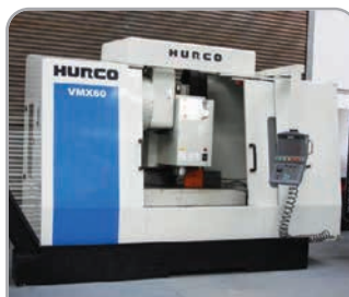
Hurco VMX60m with WinMax control, 10,000 RPM spindle, thru coolant, swarf conveyor. YOM 2011
