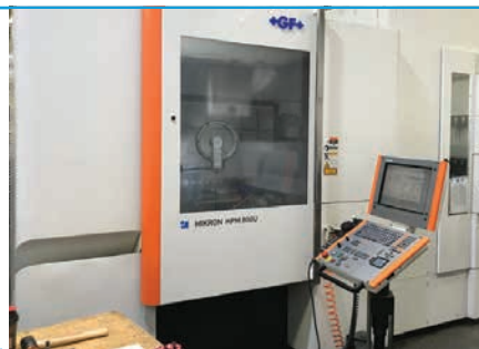
2010 MIKRON HPM 800U . Spindle taper HSK63, max workpiece size 800kg, number of axes controlled 5/5 simultaneous, spindle speed 20,000rpm, table size 500 x 631mm, 165 ATC, traverses XYZ: 800 x 800 x 550mm, machine weight 15,500kg, through-spindle coolant, swarf conveyor, touch probe
