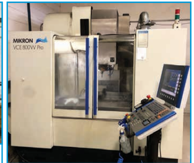
MIKRON VCE 800W Pro (2005). 14k spindle, ISO 40, 24-position T/C, scales in all axes, Heidenhain 530 control.
