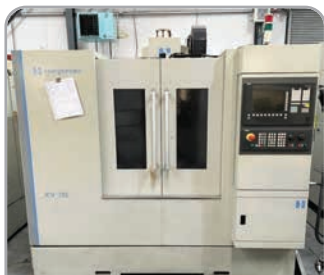
Hardinge Bridgeport XV 710 with Siemens 810D control & Shopmill, 8,000RPM BT40 spindle. Immaculate! YOM 2007
