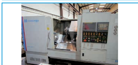
Hardinge RS51MSY CNC Lathe, with C & Y axis, sub-spindle and milling (2007)
