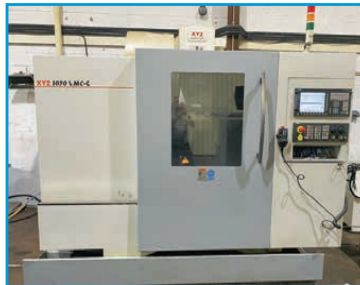
XYZ 1020 VMC Vertical Machining Centre (2012). Traverses X/Y/Z: 1,020 x 520 x 575mm, table 1,120 x 500mm, 20hp spindle motor, Siemens 828 with Shopmill control, 8,000rpm spindle, coolant, 24-station ATC, BT40 taper, 15kW, low-volt light
