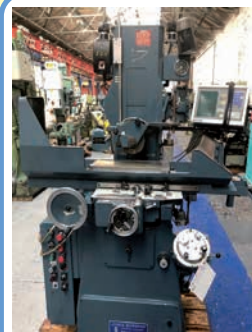
Jones & Shipman 540L power up/down, 2 axis DRO, mag chuck Email: sales@bdttools.co.uk
