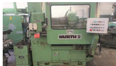
HURTH KF32a Automatic Twin Spindle Spine Milling Machine , Table size 1500 x 375mm, Horizontal travel of spindle head 400mm, Max. component length 550mm. Twin spindle index head, Hydraulic tailstocks, Arbor support, late machine. Email: sales@ronthompsonmachinery.co.uk
