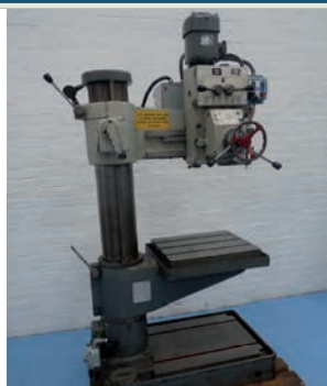
Qualters & Smith R2 24" 3MT Radial Arm Drill
