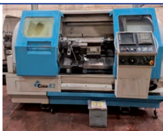
Colchester Combi K3 Slant Bed CNC Lathe Year: 2002 / FANUC 210i-T (ST3351)
