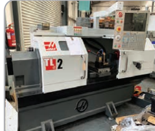
Haas TL2 with quick change tool post and holders, 8" 3-jaw chuck, coolant. YOM 2014. As new!
