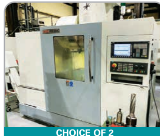
XYZ 1020 VMC with Siemens 828D control, 8,000RPM, 24-tool side-mount tool changer. YOM 2012
