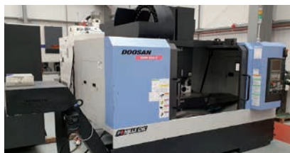
Doosan DNM 650II vertical machining centre , New 2014, Kitagawa 4th axis, Fanuc I Series, BT 40, speeds to 12000rpm, 1300 x 670mm table, X=1270 Y=670 Z=625mm 3500 cutting hours (21011) £P.O.A Email: nick@newcentury.co.uk
