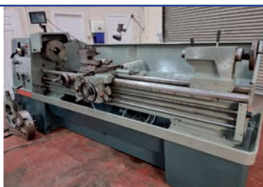
Colchester Mastiff 1400 Gap Bed Lathe 2000mm between centres (ST3371)
