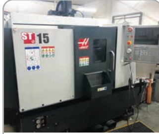
Haas ST15-TCE with power chuck, tailstock, swarf conveyor, parts catcher. YOM 2018
