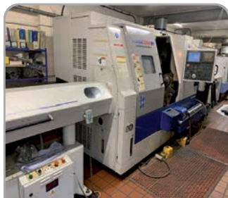
Daewoo Puma 200SY with Fanuc control, Sub Spindle, driven tools & 2 x C Axis, barfeed & swarf conveyor. YOM 2006
