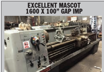
C/w 3 & 4 jaw chucks, Q'change toolpost & holders, Heavy duty steady, lo-vo-lite, Excellent slides & headstock. Original paint from new. Three months parts warranty. £POA
