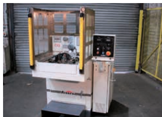
SUNNEN SSH-1680 HONE New 2018, Bore 3 - 60mm, Max Bore Length 250 mm, Spindle Speeds 250-2500rpm, Stroke speed 80-310spm C/w light guards
