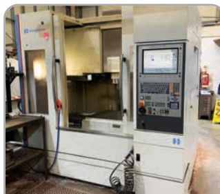
Hardinge Bridgeport XR 760 with Heidenhain i530 control, 12,000RPM direct-drive spindle, thru coolant, 4th axis probing. YOM 2008
