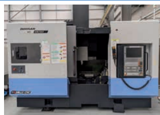
Doosan VC630 / 5AX vertical machining centre , Installed 2017, Heidenhain TNC 630i CNC full 5 axis, BT40, speeds to 12000rpm, X= 650 Y=765 Z=520mm A=150 +30 - 120 deg(20996) £P.O.A Email: nick@newcentury.co.uk
