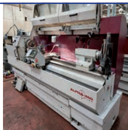
Harrison Alpha 460 Plus CNC / Manual Lathe 2000mm between centres (ST3388)
