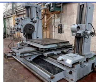
TOS W100A Horizontal Borer With End Steady / DRO / Facing Head (ST3331)
