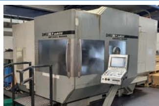
DMG DMU 80P DuoBLOCK machining centre , Heidenhain TNC 530i, 5 axis, speeds to 24000rpm, 785 x 630mm table, X=800 Y=800 Z=800 C=360 deg B= -25 deg/+ 120 deg (21013) £P.O.A Email: nick@newcentury.co.uk
