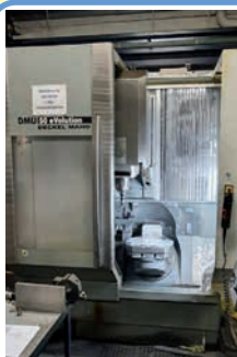
DMG DMU 50 Evolution vertical machining centre , Full simultaneous 5 axis, Heidenhain TNC 530i, SK40 taper, 18000rpm, X=500 Y= 420 Z= 380mm B=180 deg C=360 deg (21015) £P.O.A
