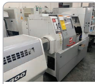
Haas SL10 with parts catcher and swarf auger, fitted with Haas Servo 300 bar feed. YOM 2004
