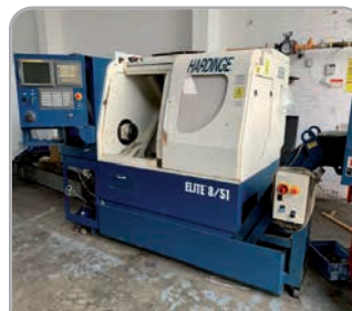
Hardinge Elite 8/52 with Fanuc control, C-axis & live tools, driven tooling package, bar feed. YOM 2003
