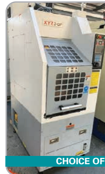
XYZ 2 OP portable VMC with ProtoTrak control, 8-tool ATC & tooling. YOM 1996
