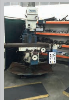
Heavy Duty Induma Vertical Mill. Table 60" x 11". ISO 40int. Two axis Anilam dro. Variable speed head. Variable & Rapid feed to table. Coolant £2,500+VAT
