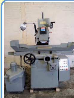
SEEDTEC YSG-618AHR Surface Grinder , (1993), Capacity 500 x 150mm, Travels 550 x 177mm, Magnetic chuck 340 x 150mm, Auto reversing saddle, Coolant and dust, Excellent condition. Email: sales@ronthompsonmachinery.co.uk
