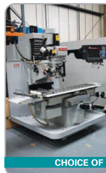
XYZ SMX 4000 with ProtoTrak SMX control, programmable spindle speeds, Traking, electronic handwheels & power. YOM 2012
