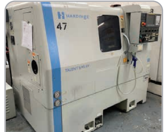
Hardinge Talent 645-SV with Fanuc control, 6" chuck, 42mm spindle. Immaculate! YOM 2006
