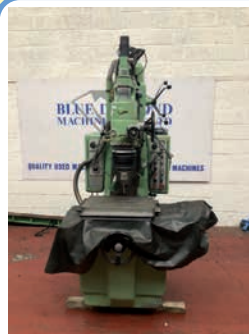
MOORE No 2 C Jig Grinder , Table 550mm x 310mm, XYZ 420 x 270 x 92mm
