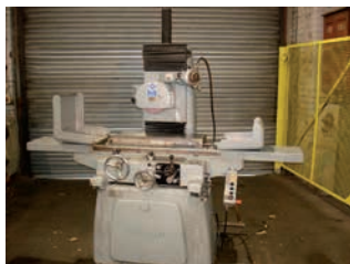
JAKOBSEN SJ16 Hydraulic Surface grinder , Capacity 800 X 300 mm Magnetic chuck 750 x 250 mm C/w Power rise & fall with incremental down feed
