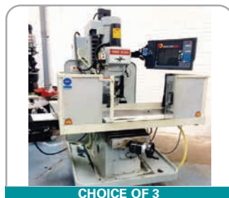
XYZ SMX 3500 with ProtoTrak SMX control, electronic handwheels, Traking & power drawbar. YOM 2013
