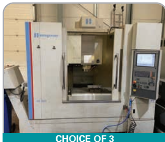
Hardinge Bridgeport XR 1000 with Heidenhain i530 control, 12,000RPM direct-drive spindle, thru coolant, 4th axis probing. YOM 2010
