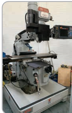
XYZ SMX 3000-3 with 3-Axis ProtoTrak SMX control, vari-speed head, ISO 40 spindle. YOM 2008
