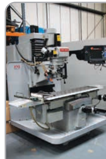
XYZ SMX 4000 with ProtoTrak SMX control, programmable spindle speeds, Traking, electronic handwheels & power. YOM 2012
