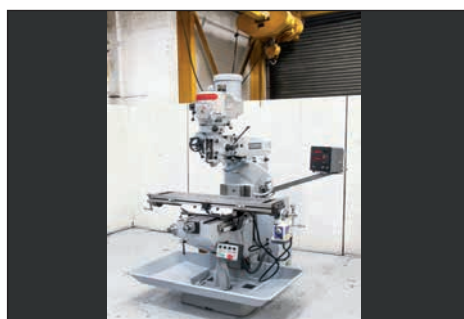
Bridgeport Turret Milling Machine 2 Axis DRO Re Ground Slideways
