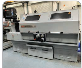
XYZ SLX 425 x 1250 with ProtoTrak SLX control, 3- & 4-jaw chucks, quick change tool post. YOM 2015
