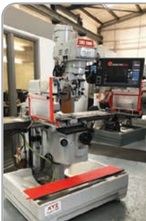
XYZ SMX 2000-2 with R8 spindle, power draw bar, DXF file reader and table guards. YOM 2016
