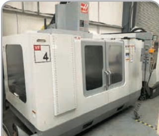
Haas VF4, 1,270mm x 508mm x 635mm movements, 8,100RPM, swarf auger. YOM 2007
