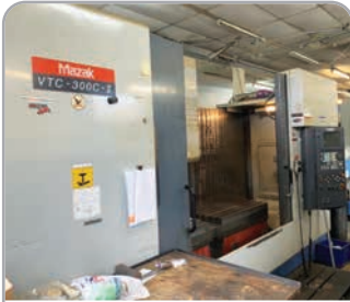
Mazak VTC 300-C Travelling Column VMC with Mazatrol PC Fusion control, 12,000RPM spindle. YOM 2004
