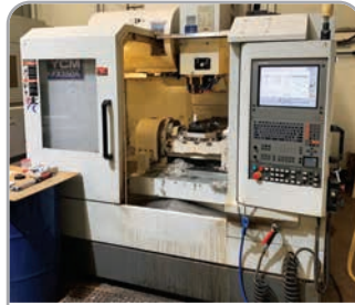
YCM FX 350A 5-Axis Machining Centre with Heidenhain i530 control, 12,000RPM, thru coolant, 60-tool ATC, glass scales & probing. YOM 2012
