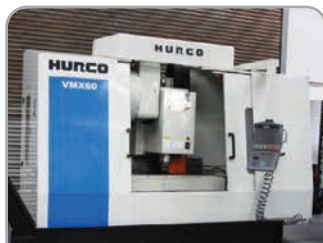
Hurco VMX60m with WinMax control, 10,000 RPM spindle, thru coolant, swarf conveyor. YOM 2011
