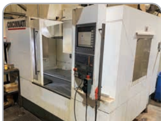
Cincinnati Lamb CFV 800i with Heidenhain i530 control, 30-tool ATC, Nikken 4th axis, 12,000RPM spindle with through coolant. YOM 2008
